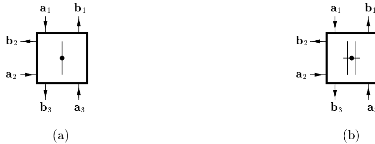
Figure 2.14: Three-port vector adaptors— (a) a vector series adaptor and (b) a vector parallel adaptor.
