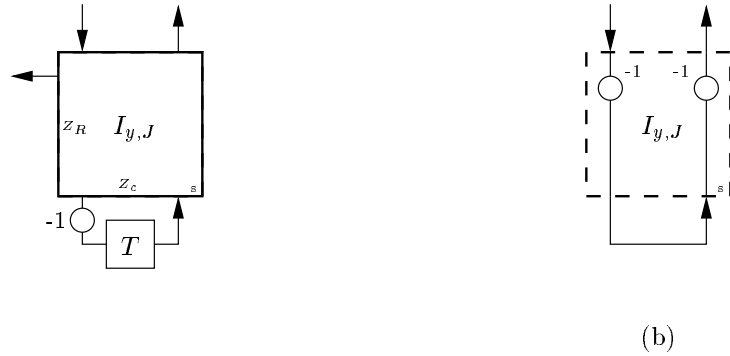
Figure 4.25: (2+1)D waveguide mesh terminations at a southern boundary, for the grid of Figure 4.23(b)—for (a) u(x, 0, t) = 0 and (b) i_y(x, 0, t) = 0 .
