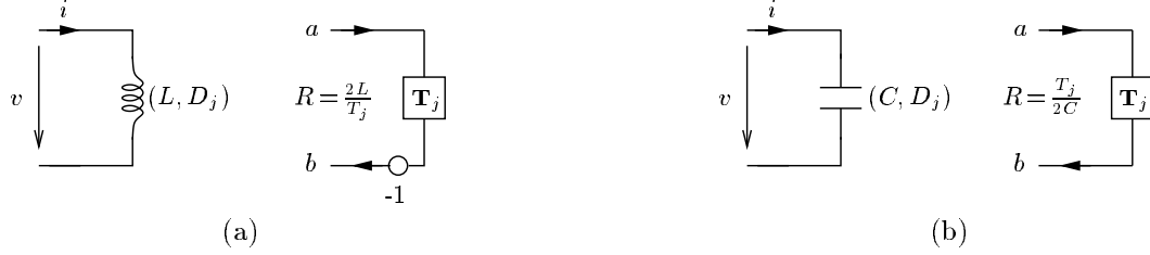
Figure 3.5: MDWD one-ports— (a) an MD inductor, with inductance L , direction t_j and its MDWD counterpart, for step-size T_j and R = 2L/T_j and (b) an MD capacitor, of capacitance C , direction t_j and its MDWD one-port, with step-size T_j and port resistance R = T_j/2C .
